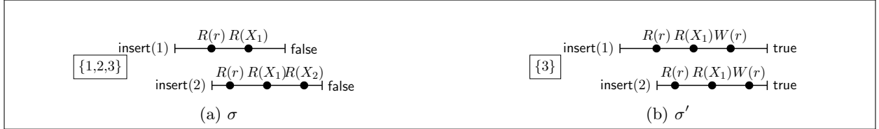
Figure 3: (a) a history of integer set (implemented as linked list or binary search tree) exporting schedule \sigma , with initial state \{1, 2, 3\} ( r denotes the root node); (b) a history exporting a problematic schedule \sigma' , with initial state \{3\} , which should be accepted by any I \in \mathcal{P} if it accepts \sigma
